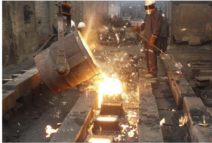
Gutter manufacturing process for the Sandhurst project
